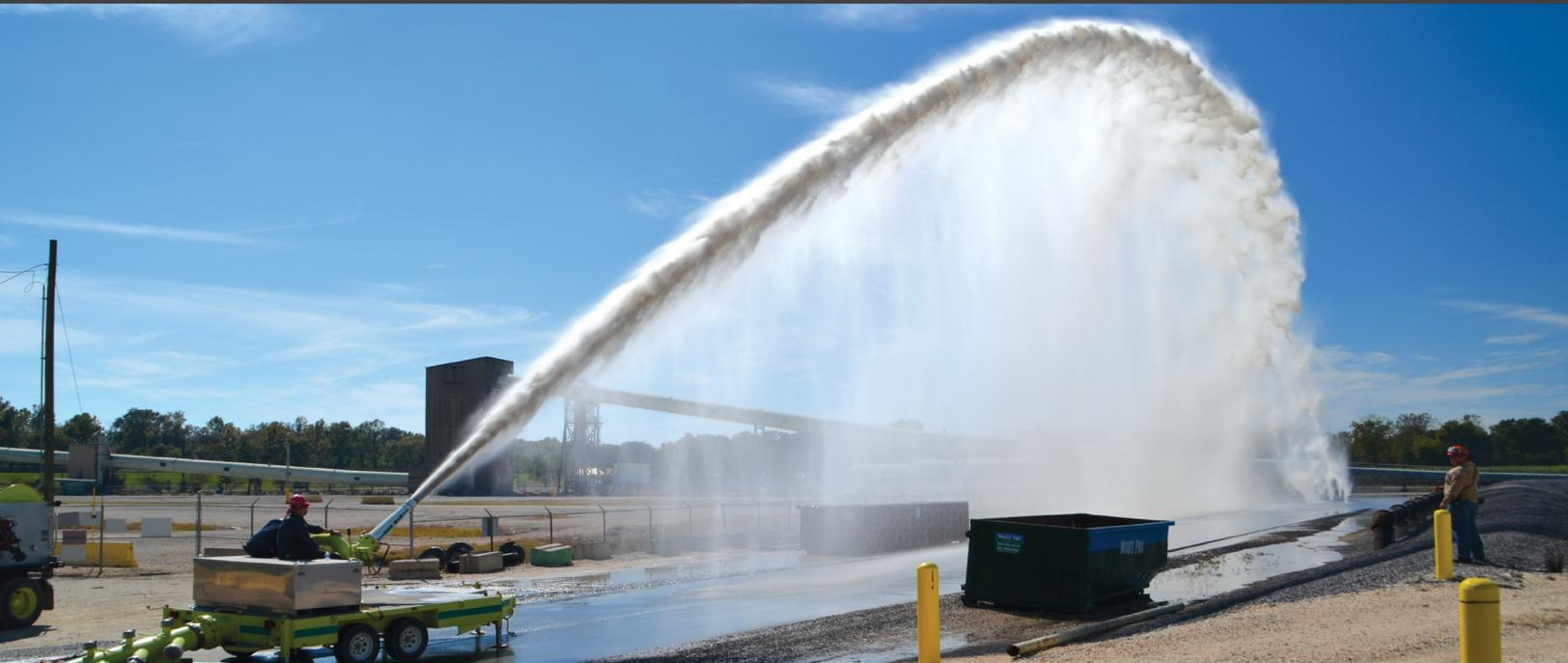
USFP pumps are designed for firefighting and high volume water supply in industrial, oil and gas, nuclear, municipal, and marine applications. The USFP High Velocity Pump is designed to exceed NFPA 1901 industrial fire pump requirements at ratings of 6000 GPM and more – the highest in the industry.
